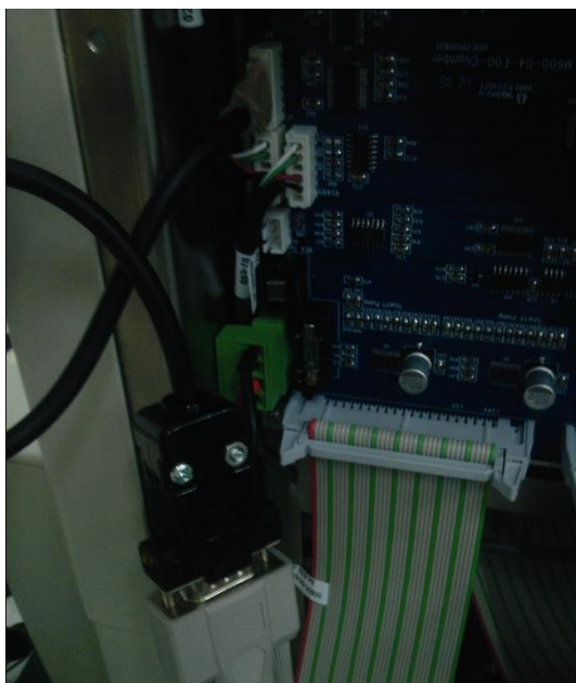
Figure B.2-9 Program Download Connection Method for Main Control Circuit Boards
