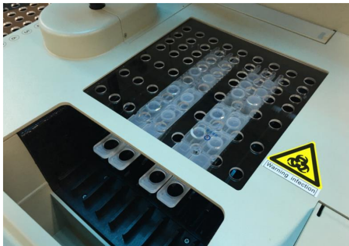
Figure 3.3-5 Reagent Tracks in the Reagent Area
