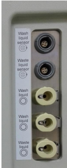
Figure 4.4-1 System Liquid and Waste Liquid connection ports
