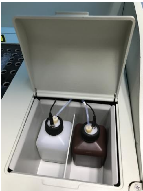
Figure 3.3-18 Starter Reagents Container inside the Analyzer
