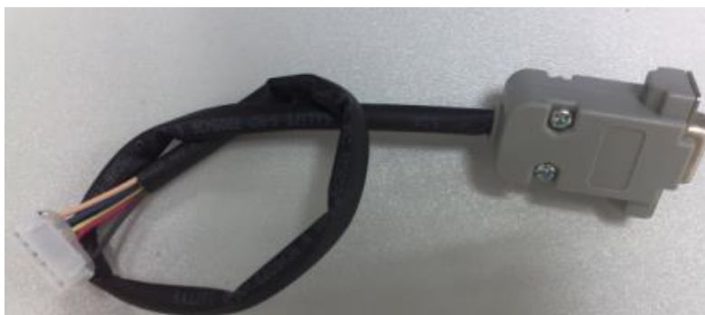
Figure B.2-4 Program Download Cable for No. 02~05 Main Control Circuit Boards
