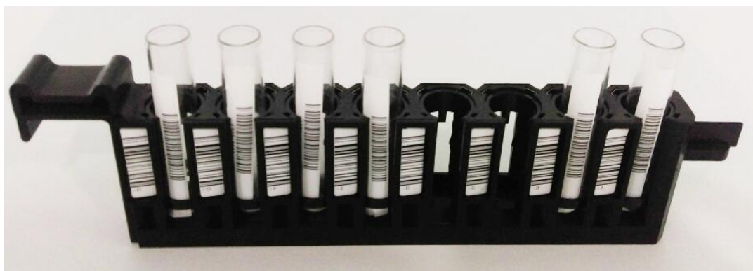
Figure 15.1-2 Sample Tube Barcodes on the Sample Rack
